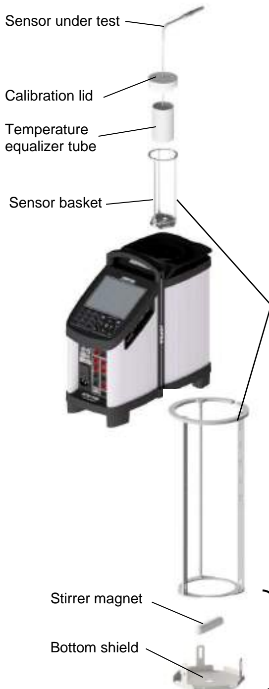
Fig. 2a Inserting the liquid bath kit RTC-168
