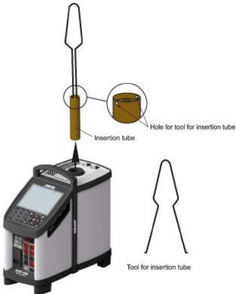
Fig. 4 Removing insertion tube
