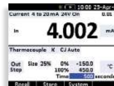
Set up span, step size, and timing. Set up and ramp times up to 999 seconds.
