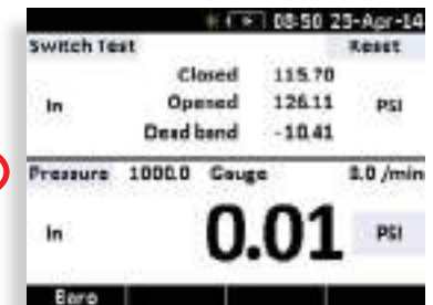
Automatic pressure switch test records automatically open, close and deadband values.
