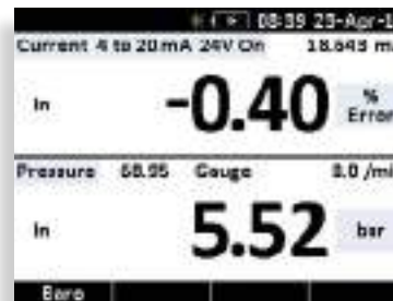
Online % calculation, fast and responsive reading, for calibration and adjustment tasks.
