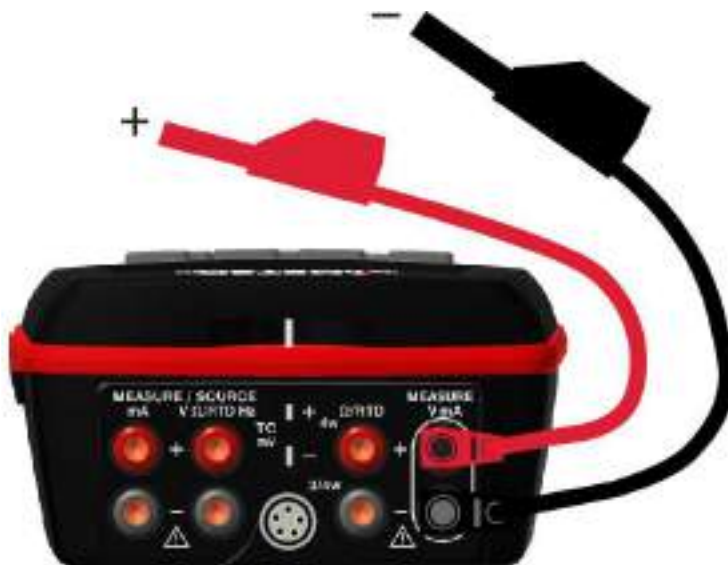
Figure 13 mA current measurement connection (upper window)
