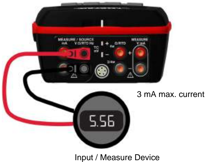
Figure 18 Connections for Testing an Output Device
