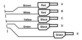
For connecting A-models to other ASM's, use 125618, cable kit.
