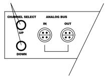
The push buttons on the back of the A-models can be used for manual channel shift. When LED 1 is flashing no channel is selected. These buttons will enable the user to operate the instrument without using a connected computer.
