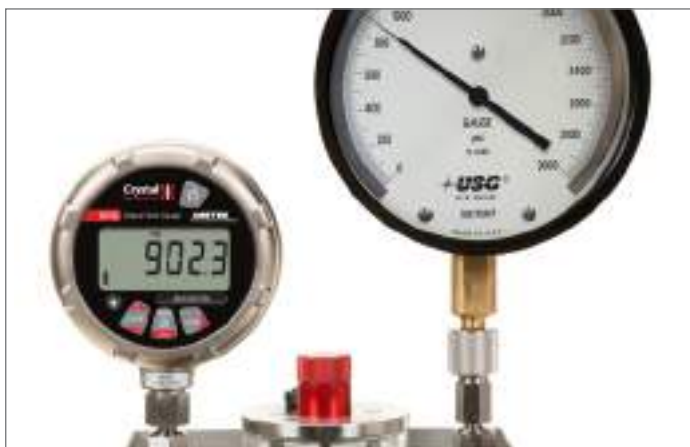
Checking the accuracy of an analog pressure gauge against the display of the reference.
