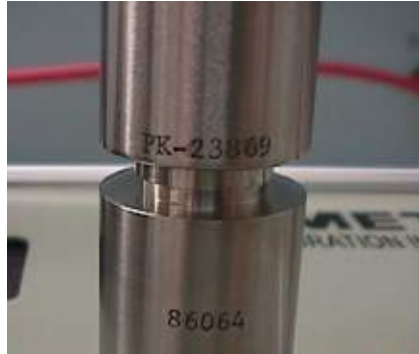
CORRECT ALIGNMENT- The serial number for the nozzle (top) aligns with the serial number of the nozzle body (bottom).
