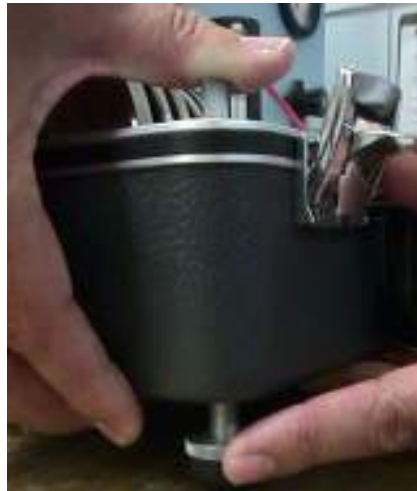
For fine adjustment, hold the bottom foot and rotate the knurled knob at the top.
