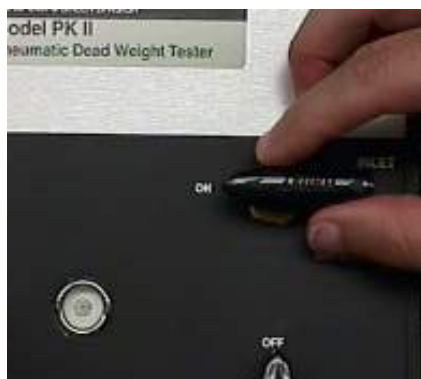
Open the INLET valve and supply pressure to the tester.
