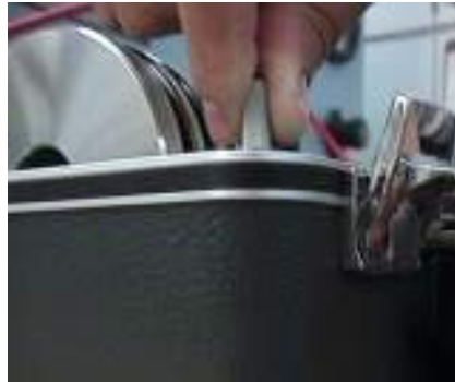
For coarse adjustment, use the knurled rod located on the top.
