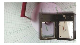
An experienced user may provide preliminary analysis on the chart output in the field, but communicating or storing the data electronically becomes possible only after a technician enters or scans the chart into a computer. This process can take days before results become available.
