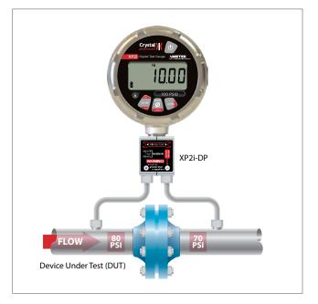
The pressure measurement accuracy of the gauge in this example is a combination of the standard accuracy statement and the static line pressure effect. The 10 psid pressure, when compared to the 100 psi full scale product used, will require the 0 to 20% of Full Scale, ± (0.02% of Full Scale) accuracy statement. The static line pressure effect relates to the lowest test pressure applied in the test, or in this case 70 psi. The pressure measurement accuracy for this test condition is as follows:
