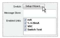
**3** Install your Red and Black test leads into the Switch Test locations as shown in the wizard. Ensure that the leads are not connected together forming a closed circuit.
