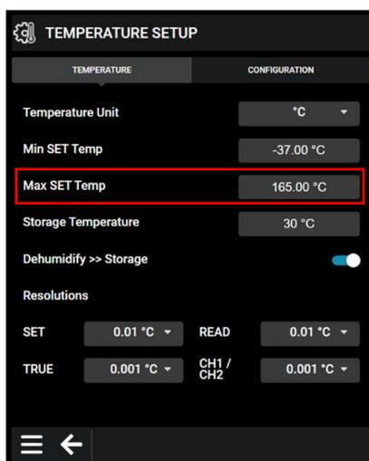
2. Let the calibrator heat and stabilize at the maximum temperature.
