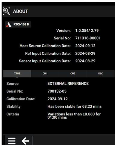
An ABOUT / STATUS summary about the calibrator type, the software version installed, the serial number and the date when it was last calibrated is displayed.
