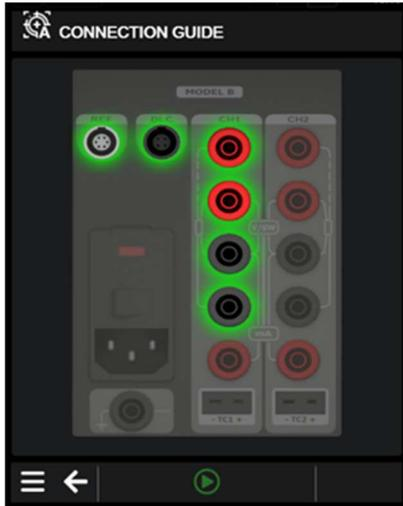
A Connection Guide is displayed, giving a graphical display of the setup and sensor connections.
