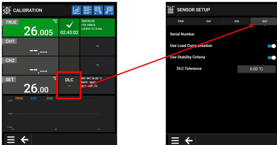
The DLC value on the Calibration screen will be read from the Intelligent Load Sensor as soon as it is connected to the DLC INPUT on the front panel (see section 4.5 fig. 7, pos. 6). The calibrator automatically reads the calibration data and serial number of the Sensor.
